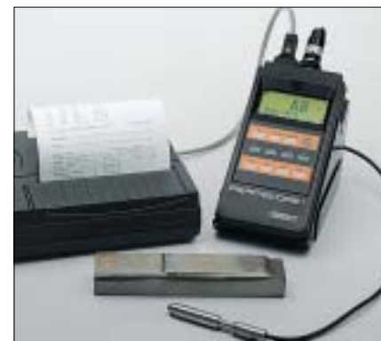
FERITSCOPE® MP30 for standardized non-destructive measurement of the ferrite content in austenitic welded products or in duplex steel.
